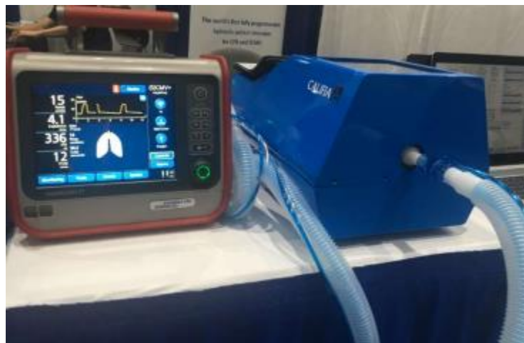
Figure 3: CALIFIA® Lung Connected to Hamilton Medical's T1 ventilator.
